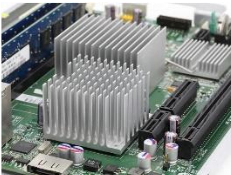
Figure 1. Heat Exchangers. (a) Electronic heat sink (b) Metal spoon in a cup of coffee (c) Platelets on a stegosaurus.
