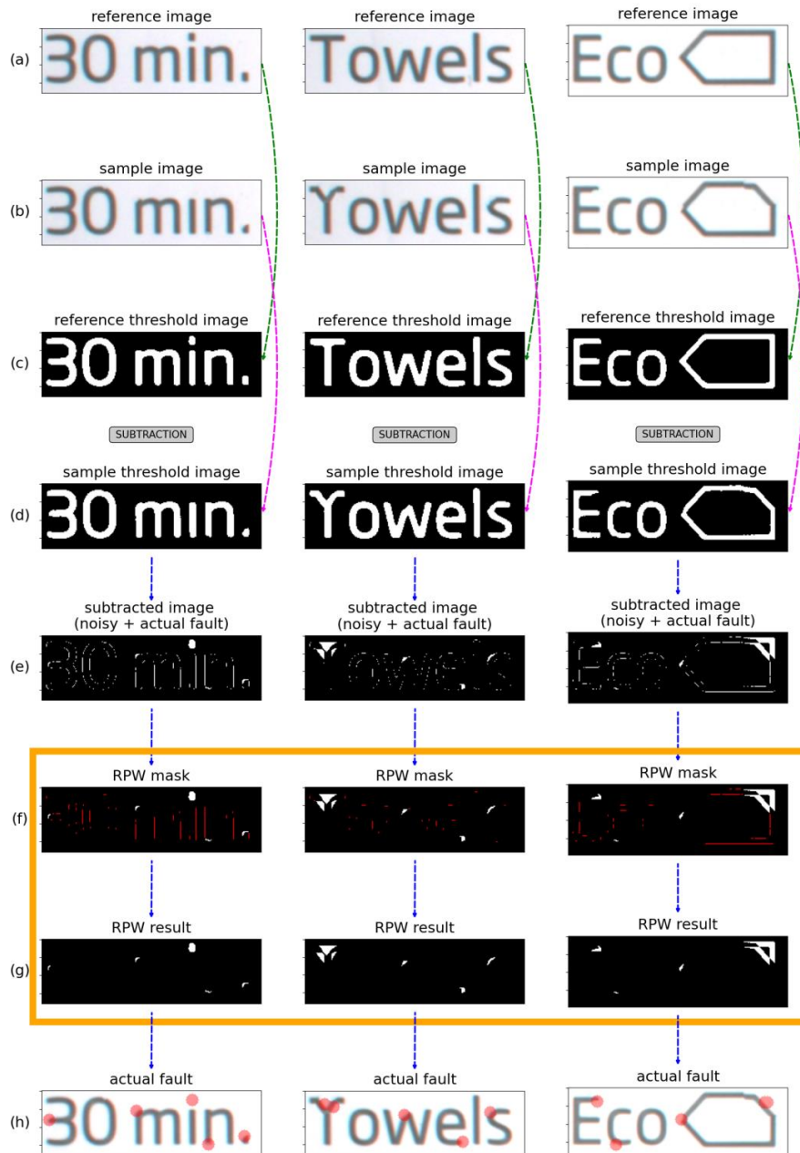
Figure 1. RPW algorithm's flow diagram is shown as initially a) reference images and b) sample images in order to compare with its related images. c) Reference and d) sample threshold images are extracted after applying many image pre-processing techniques. e) Subtracted images these are the results of subtraction process of the reference and the sample images. f) Applied RPW-mask that means detection noisy (undesired) pixels and detected pixels are pointed in red color. g) The result images of the RPW algorithms that applied on subtracted images, and also, the RPW algorithm has exposed only actual printing fault while perfectly eliminating the undesired noisy pixels. h) Exactly actual printing faults are pointed through onto sample image with small red circle
