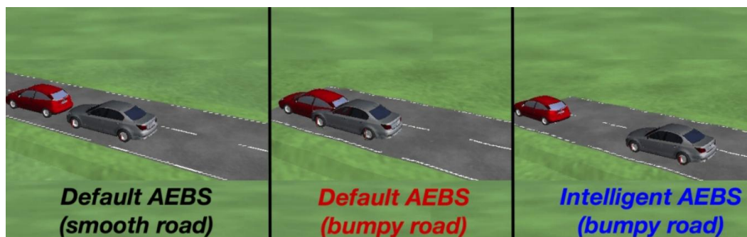
Figure 3. AEB Simulation Results on Smooth and Bumpy Roads in CarMaker
