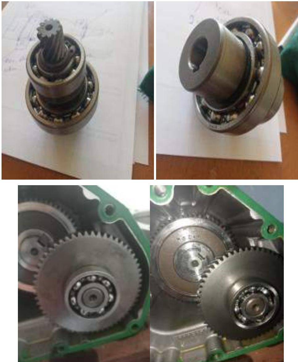
Fig. 6 Iner components: rotating shaft, bearing and helicoidal gears
