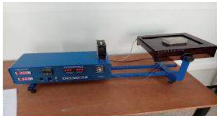
Figure 7. Conductivity meter of the mechanical engineering laboratory at the University of Bouira.
