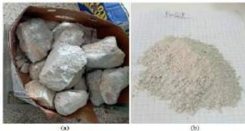
Figure 1. (a) Natural perlite in rock form before the grinding process, (b) Natural perlite reduced to powder after grinding and sieving.
