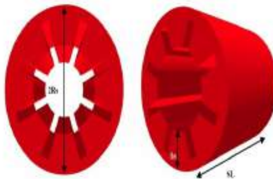
Figure 4. The Stator lamination of the SRM 8/6
