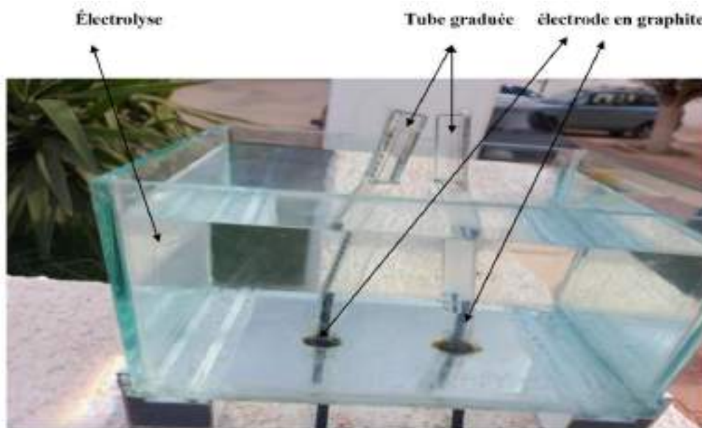
Figure 2. Elements of Water Electrolysis
