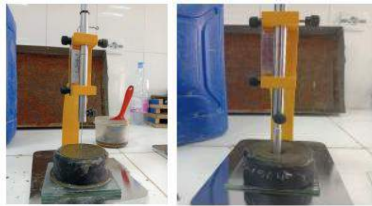
Figure 3. Consistency and setting time tests on cement paste.
