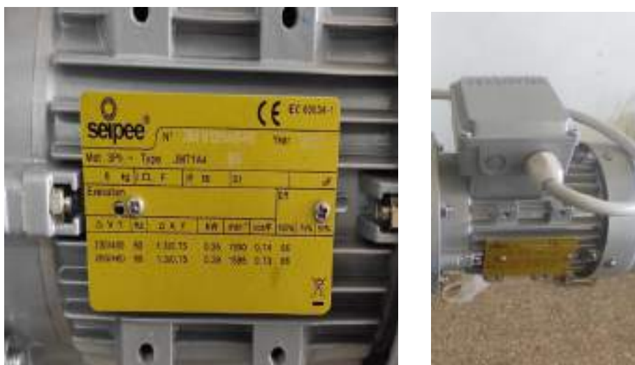
Figure 5. Motor used type SEIPEE JM71A4
